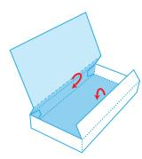
8 Fold top panel down and secure to bottom of lid.
