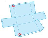
Fold front and back panels up and secure tabs to side panels.
